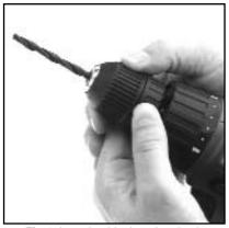
Fig 1. Inserting bits into the chuck.
